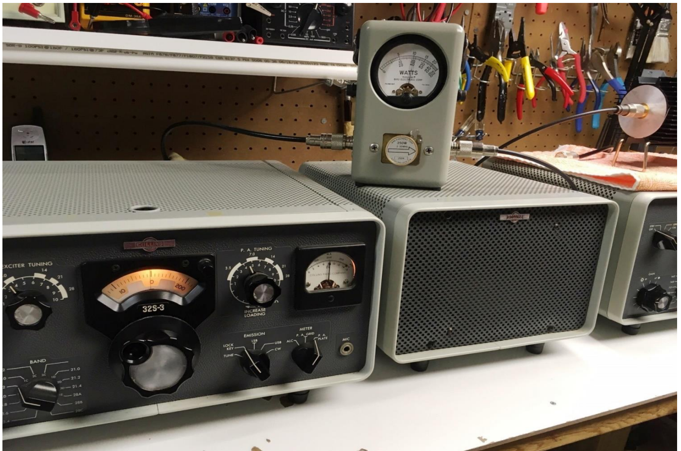
Collins 32S-3 Power Output Test on 40 Meters
