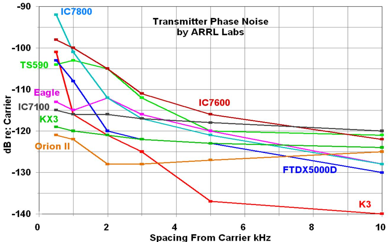
Figure 8 – Phase Noise Close To the Carrier
