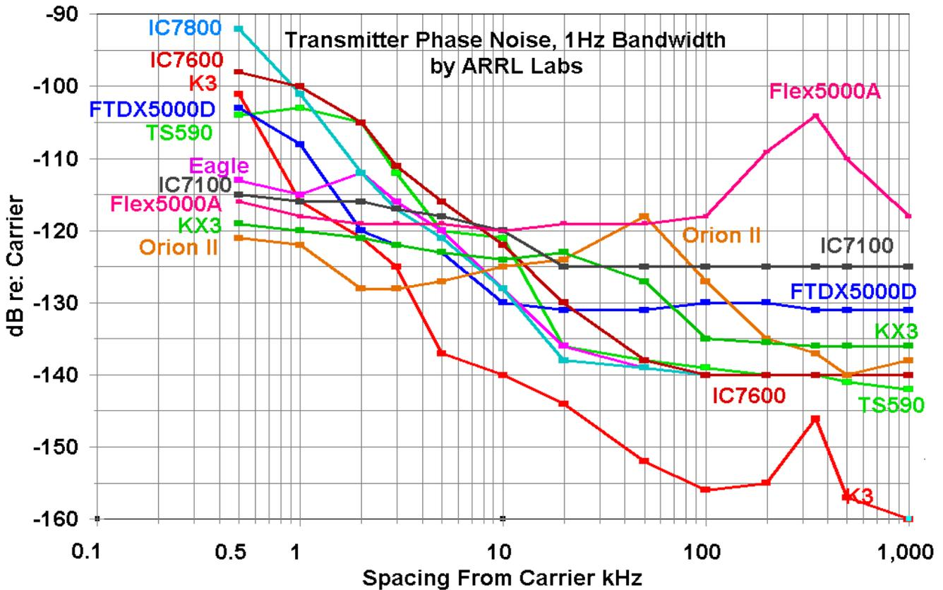
Figure 9 – Phase Noise 1 MHz Either Side of Carrier
