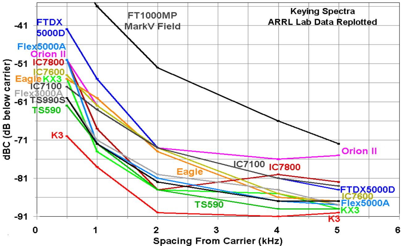
Figure 2 – The Rigs Compared For CW Spectrum
