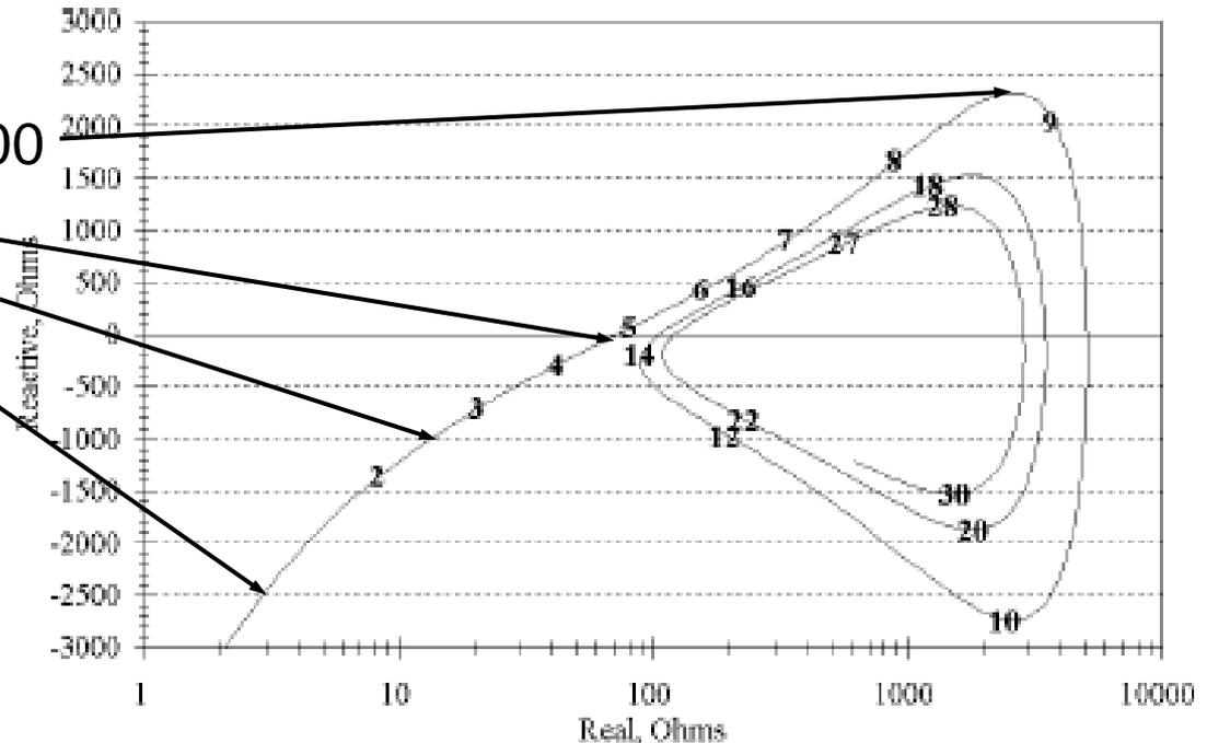
Feed-point impedance versus frequency for a theoretical 100-foot long dipole in free space, fed in the center and made of extremely thin 0.001-inch diameter wire. (Source: ARRL Antenna Book)
